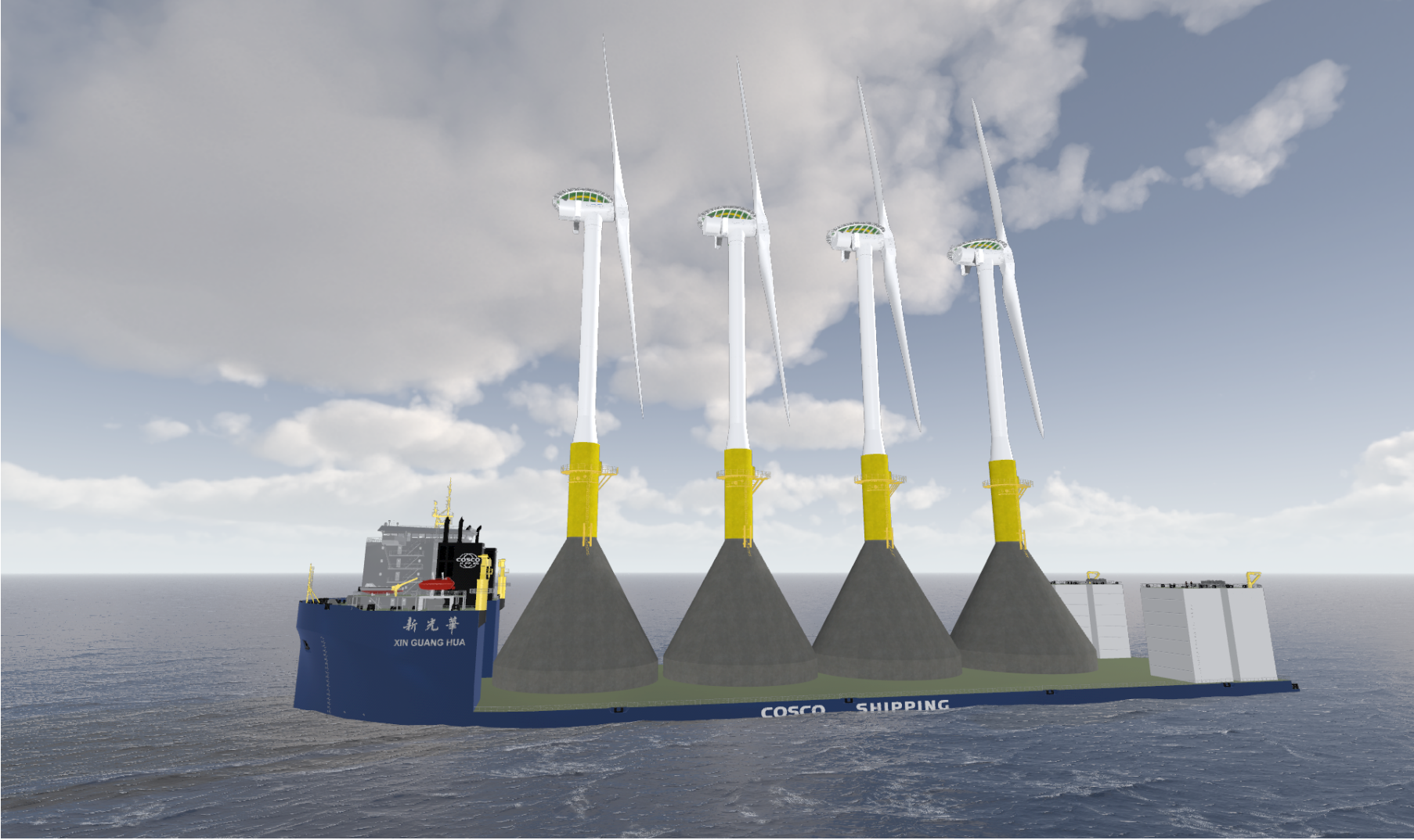
A COSCO semi-submersible heavy transport vessel delivering four complete Seawind 6 units to the offshore wind farm site
